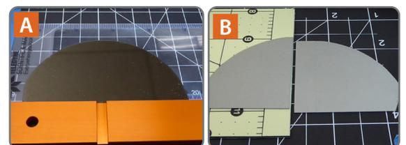
Figure 2, 2A & 2B. This shows the placement of the 4" wafer. After gently pressing the edge of the GaAs wafer, the cleave naturally occurs.
